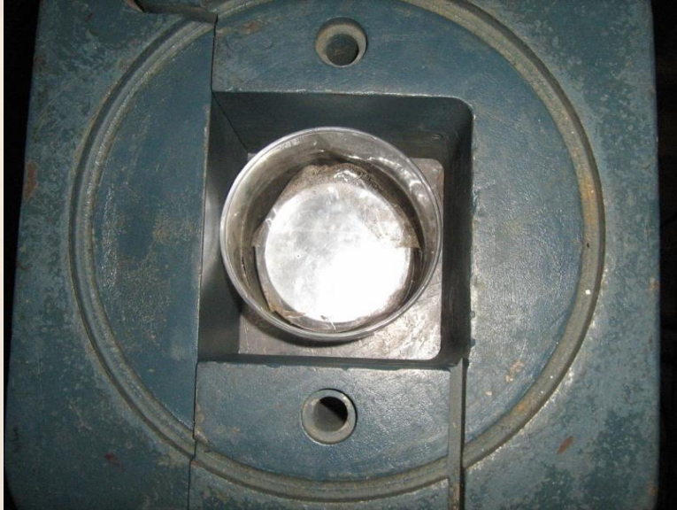
Fig(1) Top view for sediment sample in the lead shield
